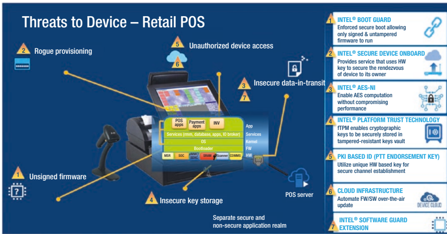
Figure 6-5. Threats to Retail POS devices with mitigation using Intel HW security building blocks
